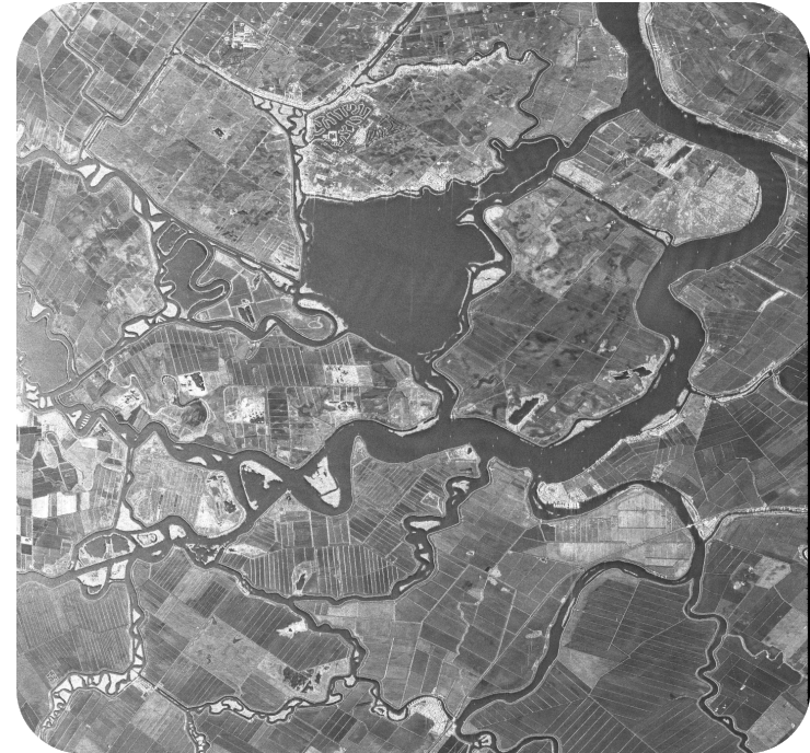
UAVSAR image of the Sacramento Delta; pixel resolution = 3m x 3m (Cathleen Jones)
