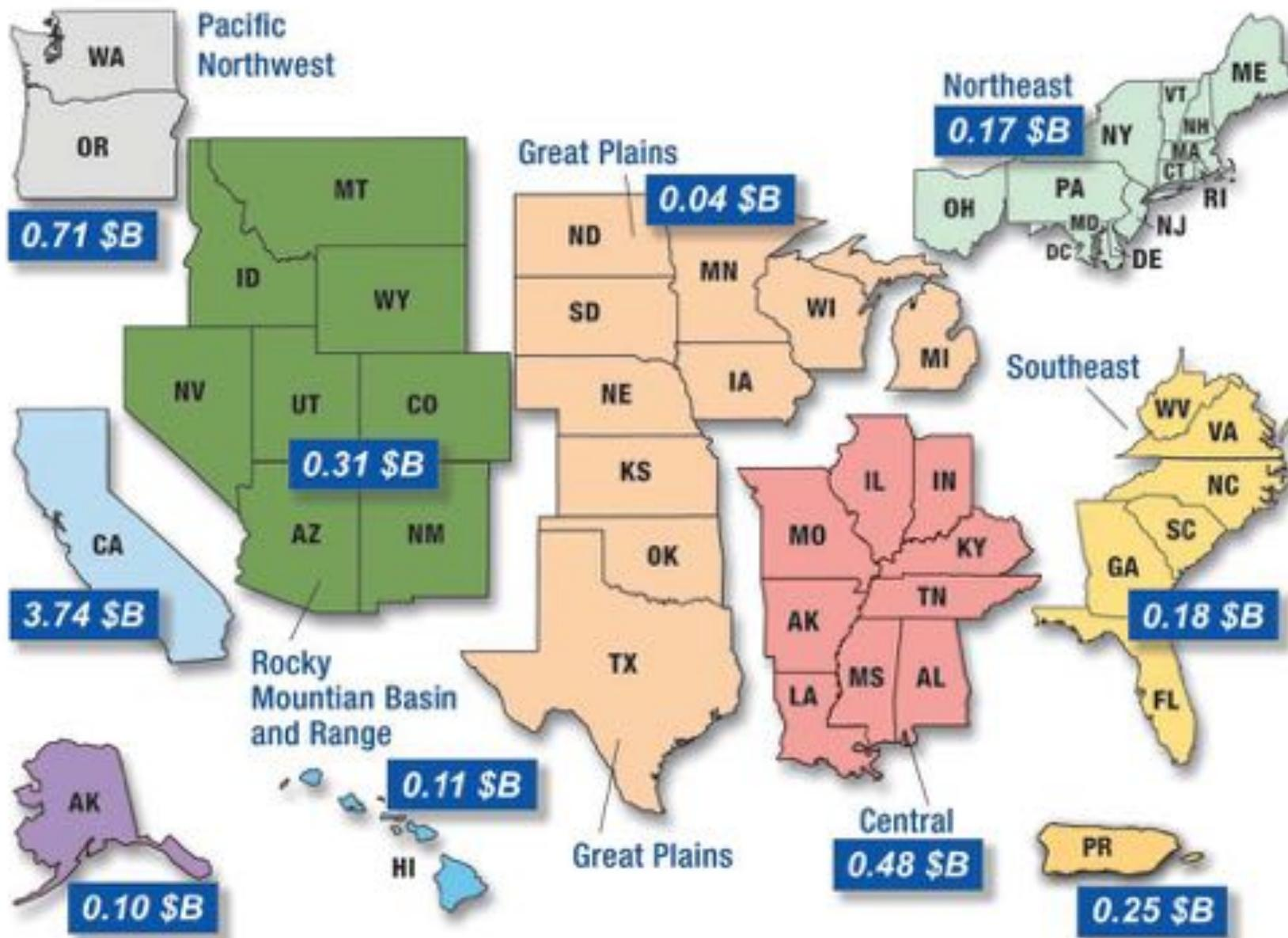
*Distribution of Average Annualized Earthquake Loss by Seismic Region*
