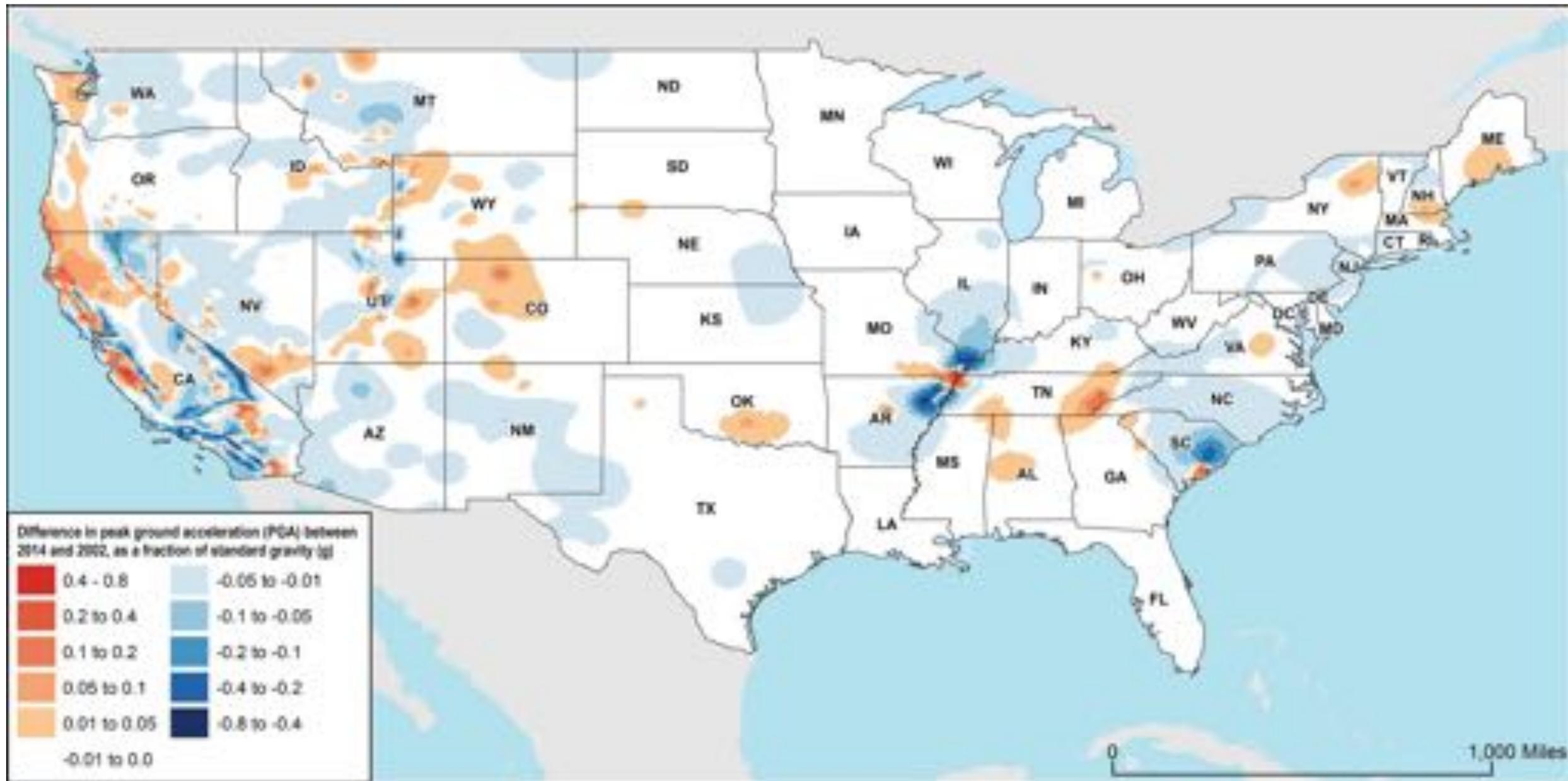
*Difference in ground motions between [2014](#) and [2002](#) USGS seismic hazard model for the 1,000-year return period*
