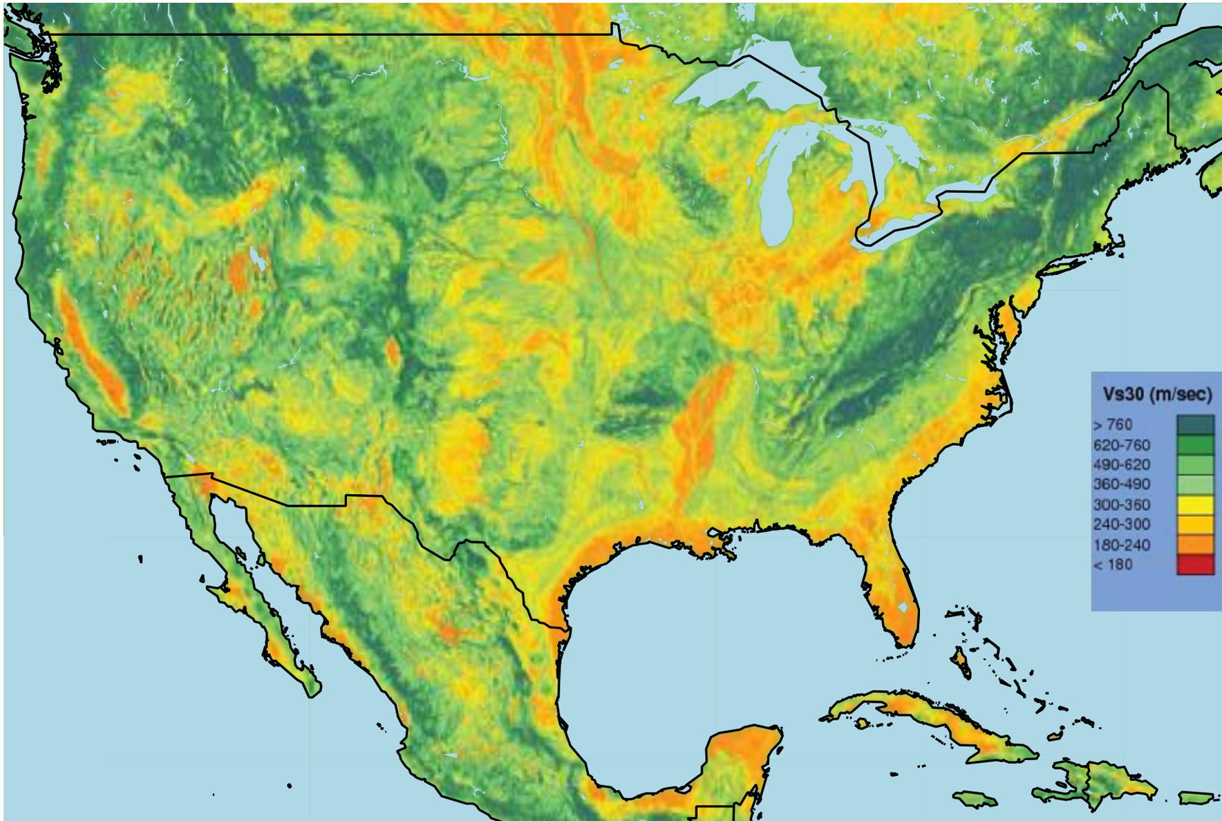
*Site categorization using Global topo-based Vs30 approximation obtained using the USGS Global Vs30 Model (<https://earthquake.usgs.gov/data/vs30/>)*
