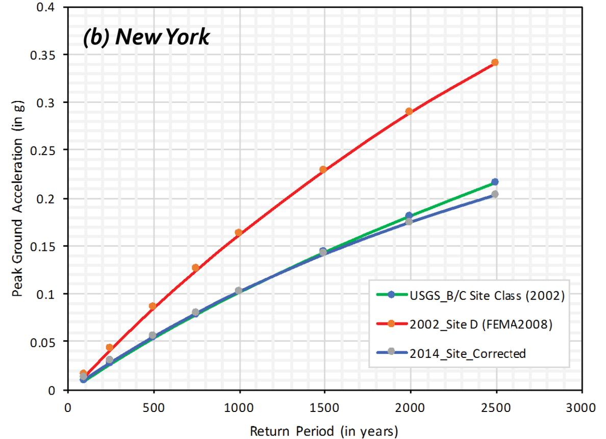
**Comparison of the hazard curves for locations in (a) Virginia and (b) New York using 2002 and 2014 USGS National Seismic Hazard Model (NSHM).**
