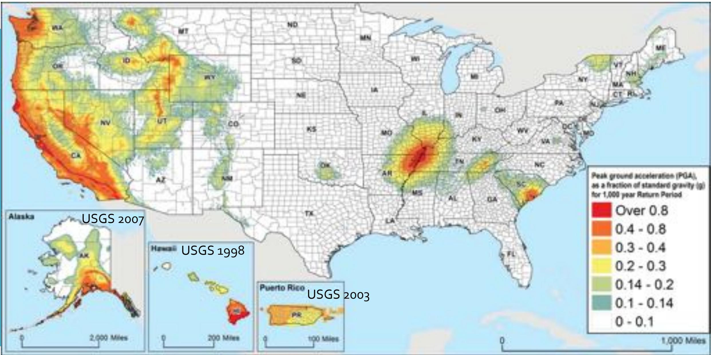
***USGS 2014 Site-Corrected Seismic Hazard Map in terms of Peak Ground Acceleration for the 1000-year Return Period***
