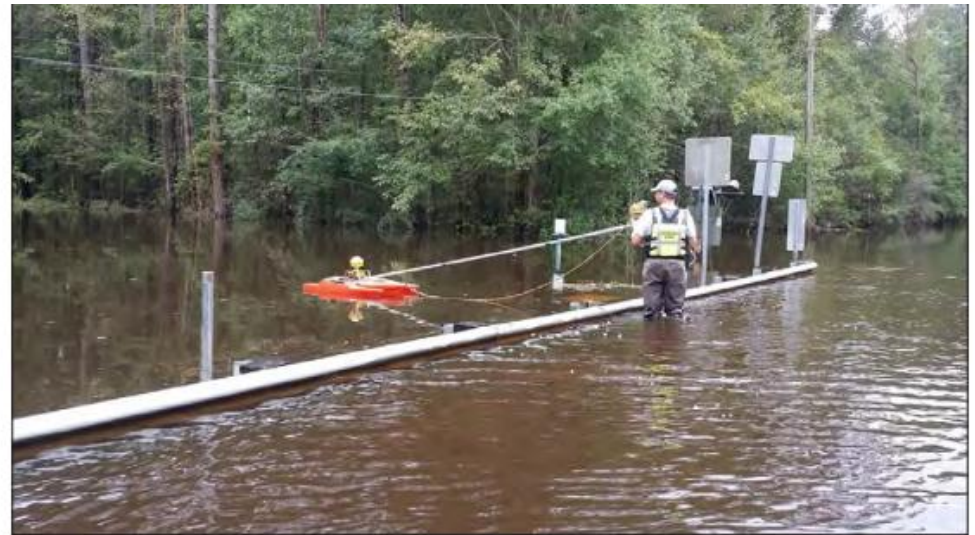
Figure 7. U.S. Geological Survey personnel making a streamflow measurement at station 02110701, Crabtree Swamp at Conway, South Carolina, using an acoustic Doppler current profiler.
