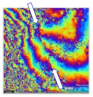
The fault trace is seen as breaks in the InSAR fringes
