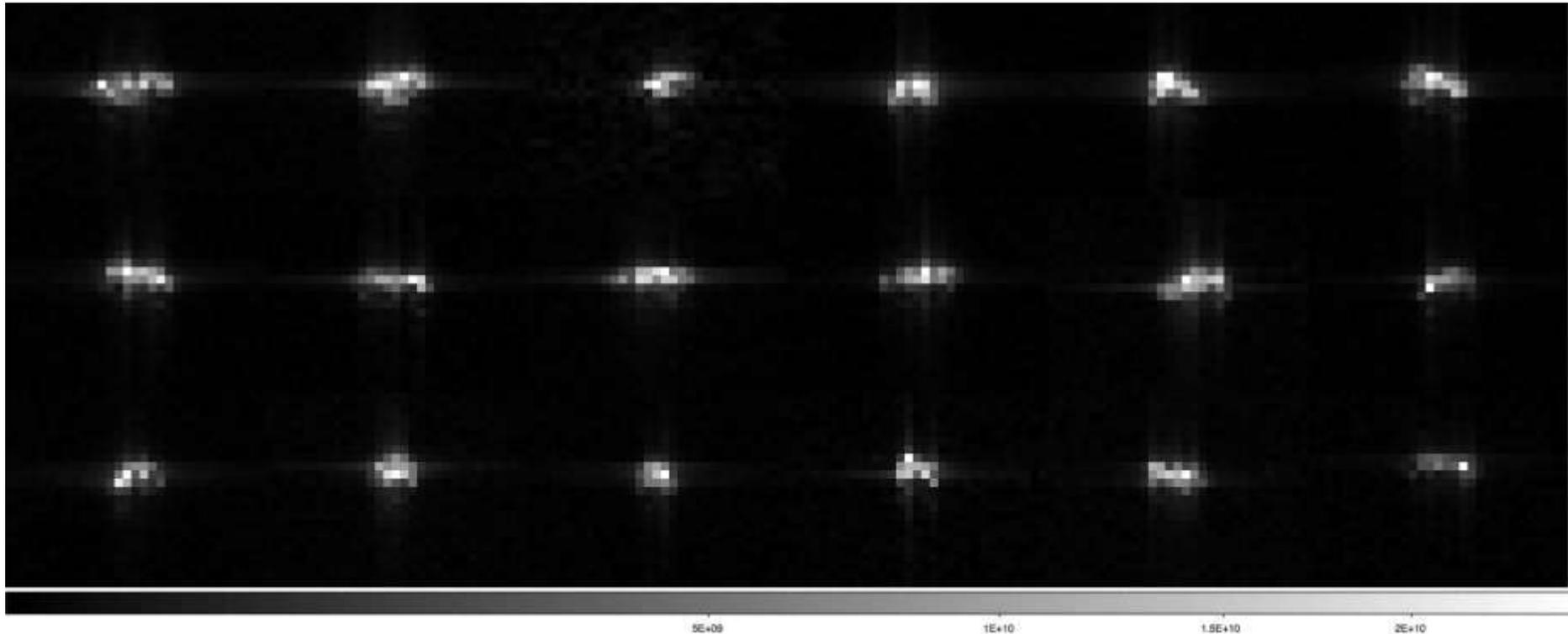
A collage of the 2012 DA14 rotation obtained with a bistatic setup at Goldstone with DSS-14 transmitting and DSS-13 receiving: Feb 16, 00:46 – 08:31 UTC. The round-trip-time (RTT) to 2012 DSS14 changed from ~0.85 s to ~2 s during observations. Each frame is 320 seconds of data integration. One full rotation is about 7 hours.
